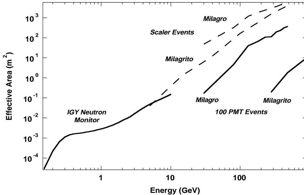
**Figure 1.** Preliminary, lower-limit effective area curves for Milagro and Milagrito, with a sea-level IGY neutron monitor for comparison. (The Milagro shower trigger is no longer set at 100 PMTs, but Milagrito shower data was recorded with a 100 PMT threshold.)
